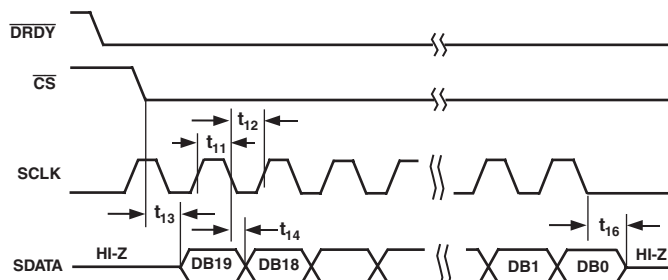
Figure 5a. SEC Mode Timing Diagram
