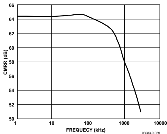
Figure 30. Analog Input CMRR vs. Frequency
