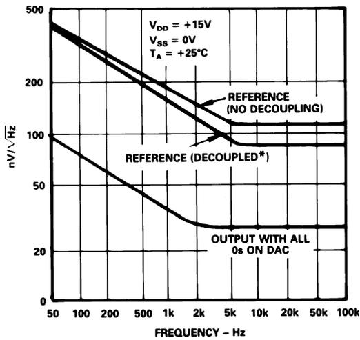
\*REFERENCE DECOUPLING COMPONENTS ARE A 200Ω RESISTOR IN SERIES WITH A PARALLEL COMBINATION OF 10μF AND 0.1μF TO GND.
