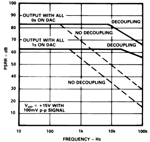
\*POWER SUPPLY DECOUPLING CAPACITORS ARE 10μF AND 0.1μF.
