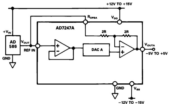
Figure 9. Bipolar Configuration
