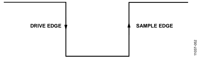
Figure 38. SPI Mode 3 SCLK Edges
