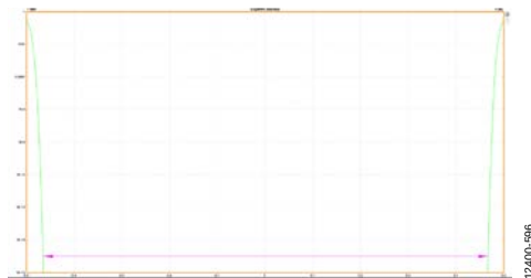
Figure 137. Bathtub, External 100Ω Terminations at 6 Gbps
