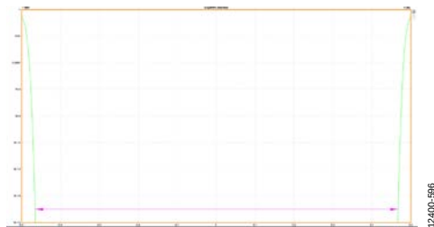
Figure 137. Bathtub, External 100Ω Terminations at 6 Gbps
