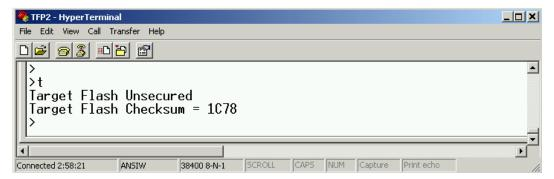
Figure 2-15: Device Checksum and Security Bit Status
