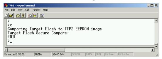
Figure 2-14: Previously Programmed Device Check with Security Bit Set
