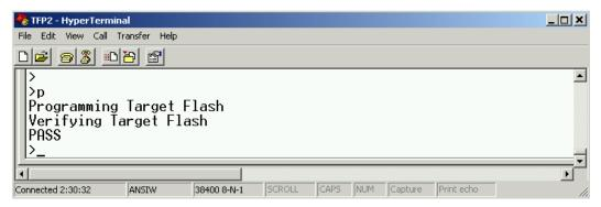
Figure 2-10: TFP2 Target Mass Erase and Program Command
