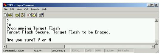
Figure 2-11: Existing Device's Security Bit Set
