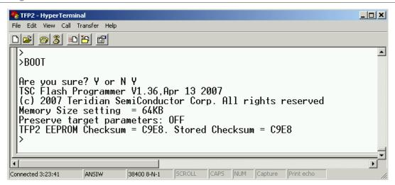
Figure 5-2: TFP2 Boot Completion
