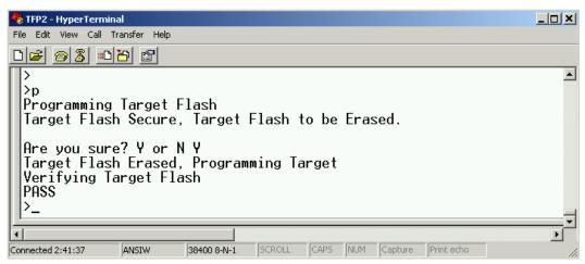
Figure 2-12: Programming Overrides Security Bit
