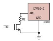
Figure 4. Dimming with an NFET and Resistor
