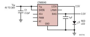
Figure 2c. Tie BIAS to an External Power Source if Neither  $V_{\text{IN}}$  Nor LPWR are Suitable
