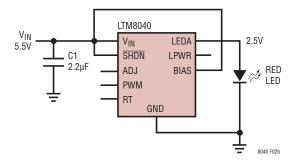
Figure 2b. BIAS May be Tied to V<sub>IN</sub> if LPWR is Below 2.6V
