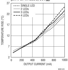
Temperature Rise vs Output Current (3.3V at 1A LEDs,  $12V_{IN}$ )
