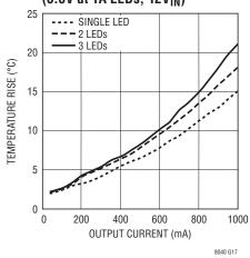
**Temperature Rise vs Output Current** (3.3V at 1A LEDs, 36V<sub>IN</sub>)
