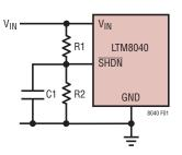
Figure 1. Undervoltage Lockout
