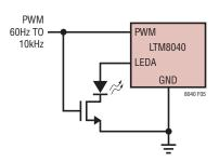
Figure 5. Dimming Using PWM Signal
