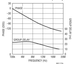
Figure 16. Modified Filter Configuration Using a Resistor Between Summing Nodes ( $f_{-3dB} = 10MHz$ )
