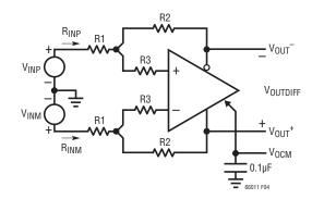
Figure 4. Input Impedance
