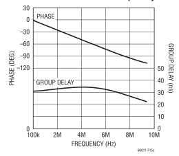
Figure 15. Modified Filter Configuration Using a Resistor Between Summing Nodes ( $f_{-3dB} = 7.5$ MHz)
