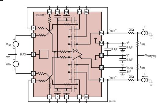
Figure 1. DC Test Circuit
