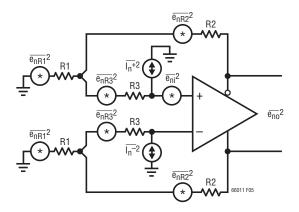
Figure 5. Differential Noise Model of the LTC6601
