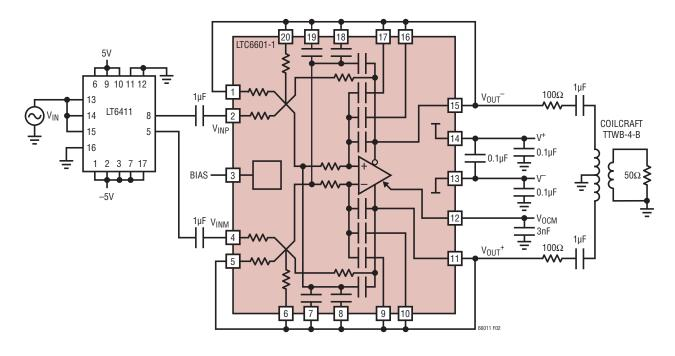
Figure 2. AC Test Circuit (Frequency Response Testing)
