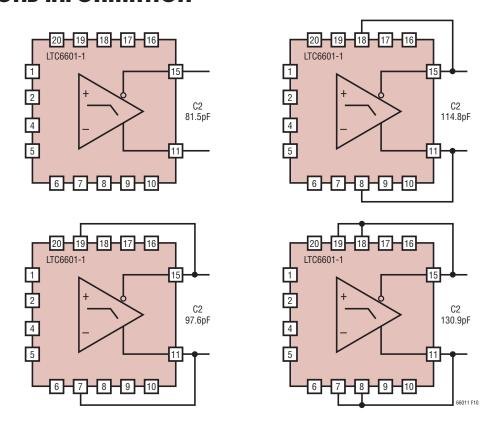
Figure 10. Pin-Strap Hookup for a Particular C2
