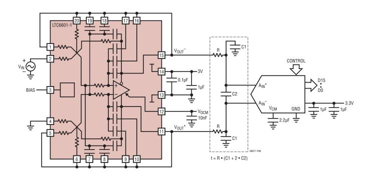
Figure 6. Interfacing the LTC6601 to A/D Converters
