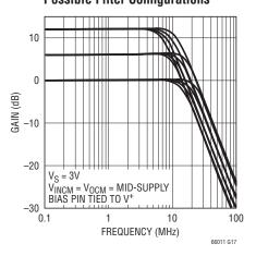
Low Power Mode Frequency Response of 12 Possible Filter Configurations
