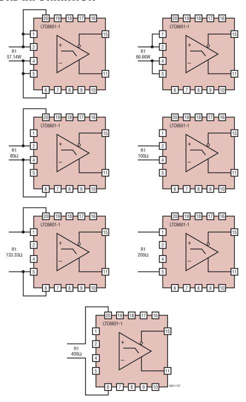
Figure 7. Pin-Strap Hookup for a Particular R1
