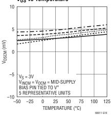
Low Power Common Mode V<sub>OS</sub> vs Temperature
