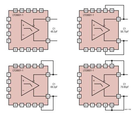
Figure 9. Pin-Strap Hookup for a Particular C1
