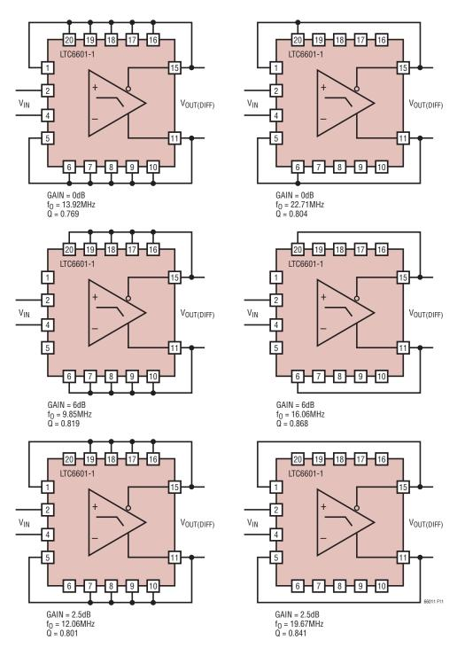
Figure 11. Basic 2nd Order Filter Configurations
