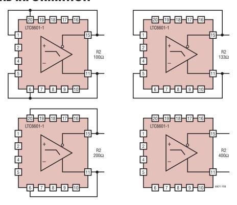
Figure 8. Pin-Strap Hookup for a Particular R2
