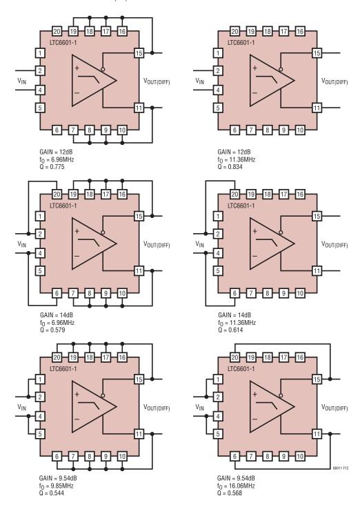
Figure 12. Basic 2nd Order Filter Configurations
