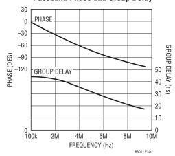
Figure 14. Modified Filter Configuration Using a Capacitor and a Resistor Between Summing Nodes ( $f_{-3dB} = 5MHz$ )
