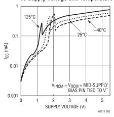
Low Power Mode Supply Current vs Supply Voltage and Temperature
