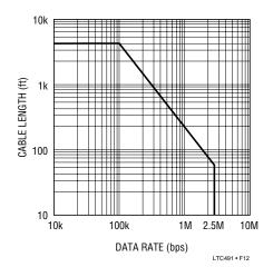
Figure 12. Cable Length vs Data Rate
