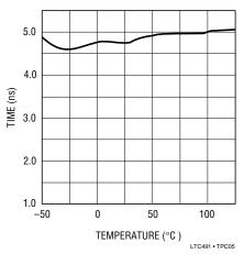
Receiver |t<sub>PLH</sub> t<sub>PHL</sub> | vs Temperature
