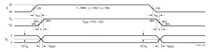
Figure 5. Driver Propagation Delays
