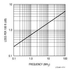
Figure 11. Attenuation vs Frequency for Belden 9481
