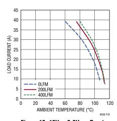
Figure 18. 12V<sub>IN</sub>, 3.3V<sub>OUT</sub> Derate Curve
