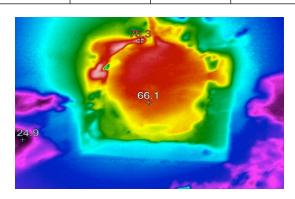
Figure 8. The Two Images Show the LTM4636 Operating at 1V at 40A and 3.3V at 35A from a 12V Input. Both Images Reflect Only a 40°C to 45°C Rise Above Ambient at Full Load Current with 200LFM.
