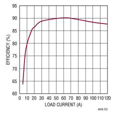
Figure 25. Efficiency, 12V to 0.9V at 120A
