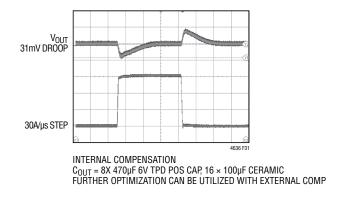
Figure 31. 12 to 0.9V 30A/µs Load Step
