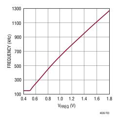
Figure 3. FREQ Voltage to Switching Frequency
