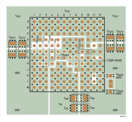
Figure 19. Recommended PCB Layout
