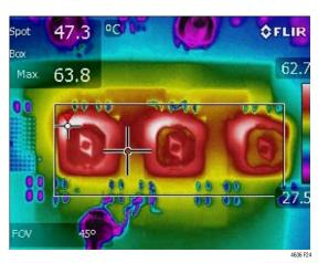
Figure 24. Thermal Plot, 12V to 0.9V at 120A, 400LFM Air Flow
