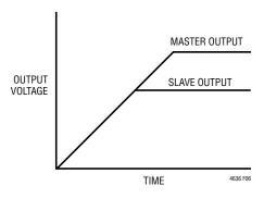
Figure 6. Output Voltage Coincident Tracking Characteristics
