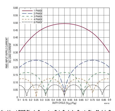
Figure 2. Normalized Input RMS Ripple Current vs Duty Cycle for One to Six μModule Regulators (Phases)
