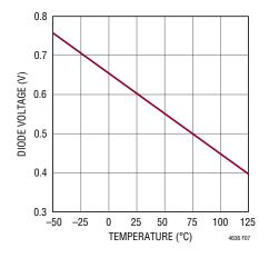
Figure 7. Diode Voltage  $V_D$  vs Temperature  $T(^{\circ}C)$
