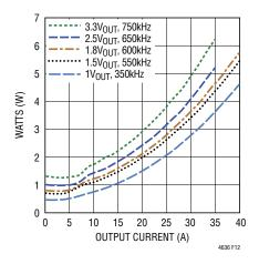
Figure 10. 5V Input Power Loss Curves
