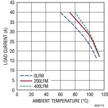
Figure 13. 5V<sub>IN</sub>, 1V<sub>OUT</sub> Derate Curve
