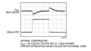
Figure 26. 12V to 0.9V 30A/µs Load Step
