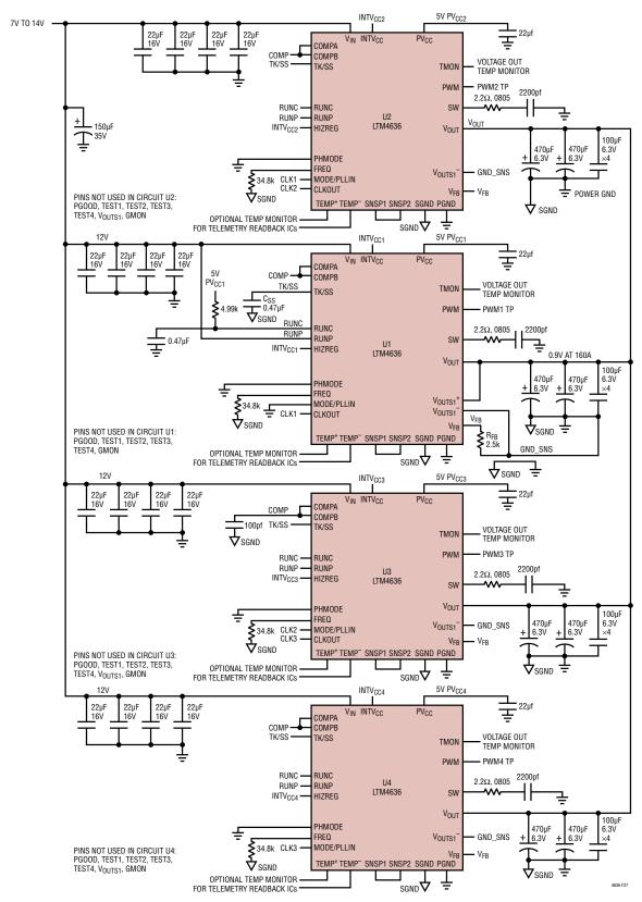
Figure 27. Four Phase 0.9V at 160A Design
