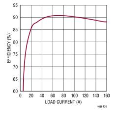
Figure 30. Efficiency, 12V to 0.9V at 160A
