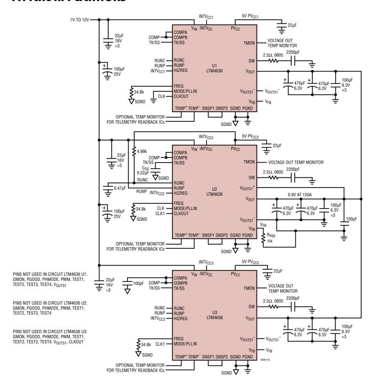
Figure 22. 3-Phase 0.9V at 120A with Protection
