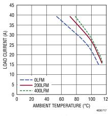
Figure 15.  $5V_{IN}$ , 1.5 $V_{OUT}$  Derate Curve
