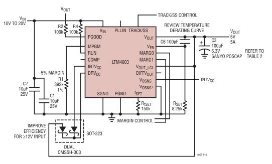
Figure 16. 5V at 5A Design Without Differential Amplifier
