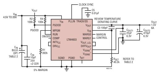
Figure 18. Typical 4.5V to  $_{20VIN}$ , 1.5V at 6A Design
