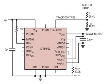
Figure 5. Coincident Tracking Schematic
