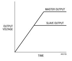
Figure 6. Coincident Output Tracking Characteristics
