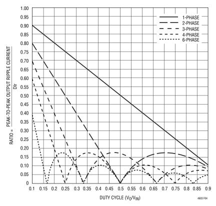
Figure 4. Normalized Output Ripple Current vs Duty Cycle, DIr =  $V_0T/L_1$
