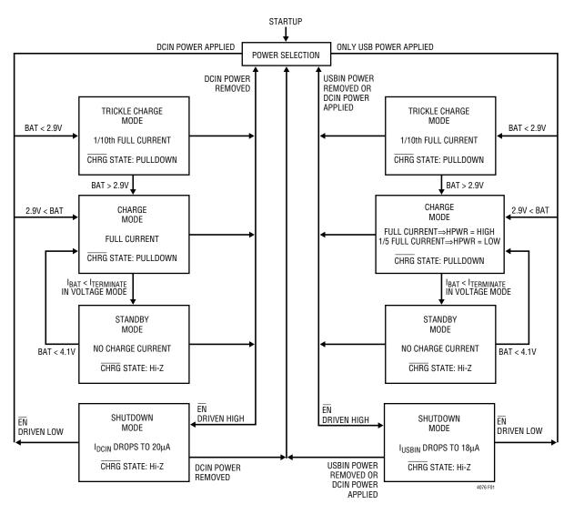
Figure 1. LTC4076 State Diagram of a Charge Cycle
