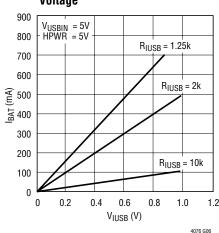
Charge Current vs IUSB Pin Voltage
