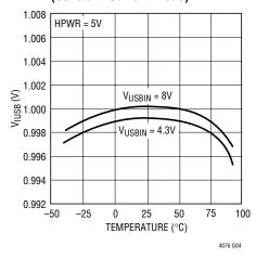
IUSB Pin Voltage vs Temperature (Constant-Current Mode)
