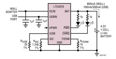
Figure 3. Full Featured Dual Input Charger Circuit
