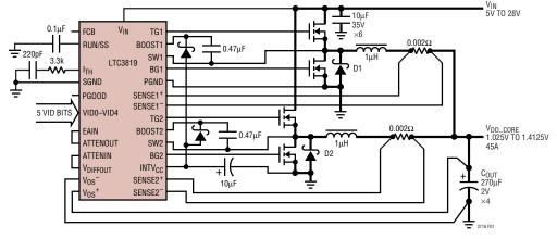
Figure 1. High Current Dual Phase Step-Down Converter
