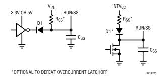
Figure 5. RUN/SS Pin Interfacing
