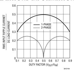
Figure 4. Normalized RMS Input Ripple Current vs Duty Factor for 1 and 2 Output Stages
