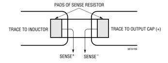
Figure 8. Proper Current Sense Connections
