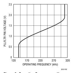
Figure 2. Operating Frequency vs V<sub>PLLFLTR</sub>
