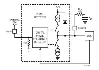
Figure 6. Phase-Locked Loop Block Diagram
