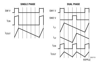
Figure 10. Single and 2-Phase Current Waveforms
