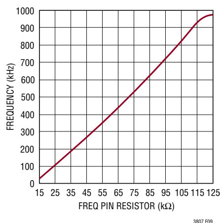
Figure 9. Relationship Between Oscillator Frequency and Resistor Value at the FREQ Pin
