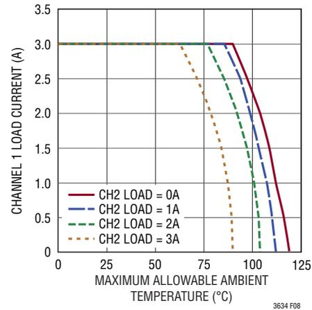
Figure 8. Temperature Derating Curve for DC1708 Demo Circuit
