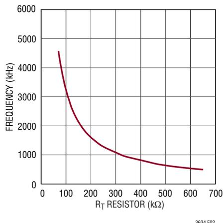
Figure 2. Switching Frequency vs R<sub>T</sub>
