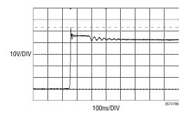
Figure 6. Good Snubber Diode Limits SW Pin Voltage
