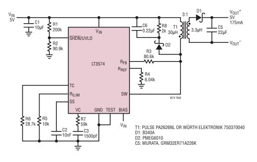
Low Input Voltage 5V Isolated Flyback Converter
