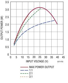
Figure 3. Output Power for 12V Output
