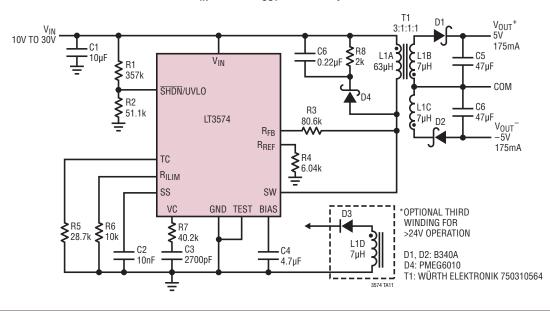
10V to  $30V_{IN}$ , +5V/–5V<sub>OUT</sub> Isolated Flyback Converter
