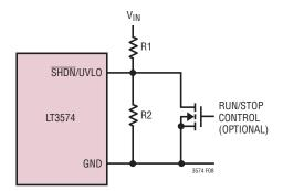
Figure 8. Undervoltage Lockout (UVLO)
