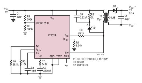
5V Isolated Flyback Converter Using Coupling Inductor
