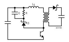
Figure 9. RCD Snubber in a Flyback Converter
