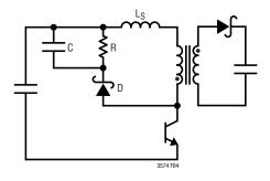
Figure 4. RCD Clamp
