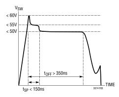
Figure 5. Maximum Voltages for SW Pin Flyback Waveform
