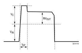
Figure 10. Typical Switch Node Waveform
