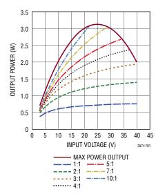
Figure 1. Output Power for 3.3V Output
