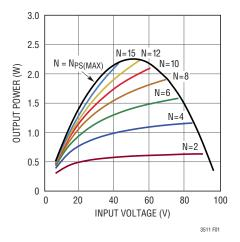
Figure 1. Output Power for 3.3V Output
