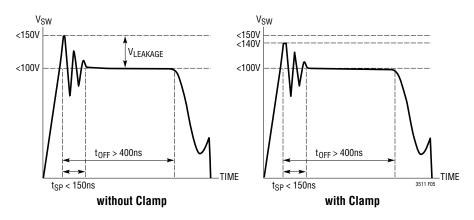
Figure 5. Maximum Voltages for SW Pin Flyback Waveform
