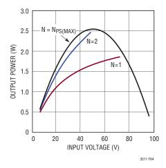
Figure 4. Output Power for 24V Output
