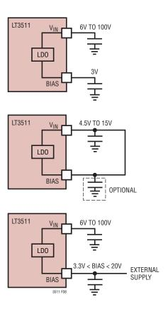
Figure 8. BIAS Pin Configurations
