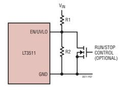
Figure 7. Undervoltage Lockout (UVLO)
