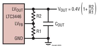
Figure 2. Programming a VLDO Regulator's Output Voltage
