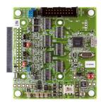
When connected to a DC9003A-B Evaluation/Development Mote, the **DC9006 Eterna interface card** provides a USB connection for both power and software access to the mote API UART port. The DC9006 comes with a DC9004 adapter card (not pictured) enabling the DC9006 to connect to the 10-pin programming and CLI header recommended for customer designs. Please see www.linear.com/ solutions/3102 for more details.
