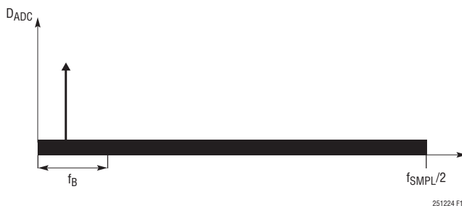
Figure 15. Frequency Spectrum of SAR ADC Core Output
