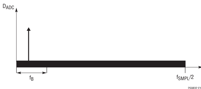
Figure 15. Frequency Spectrum of SAR ADC Core Output
