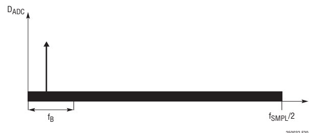
Figure 20. Frequency Spectrum of SAR ADC Core Output
