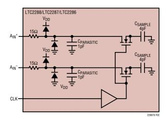
Figure 2. Equivalent Input Circuit
