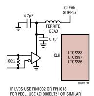
Figure 12. CLK Drive Using an LVDS or PECL to CMOS Converter
