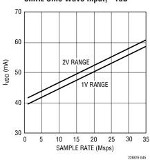
LTC2286: I<sub>OVDD</sub> vs Sample Rate, 5MHz Sine Wave Input, -1dB, O<sub>VDD</sub> = 1.8V
