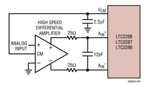
Figure 4. Differential Drive with an Amplifier
