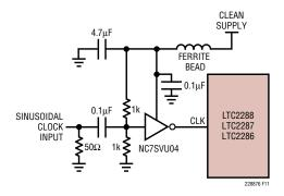
Figure 11. Sinusoidal Single-Ended CLK Drive
