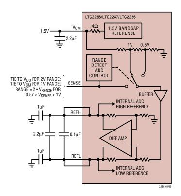
Figure 9. Equivalent Reference Circuit
