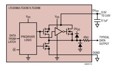
Figure 14. Digital Output Buffer
