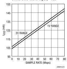
LTC2288:  $I_{OVDD}$  vs Sample Rate, 5MHz Sine Wave Input, -1dB,  $O_{VDD}$  = 1.8V
