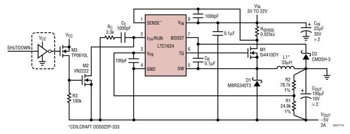
Figure 15. Inverting -5V/2A Converter
