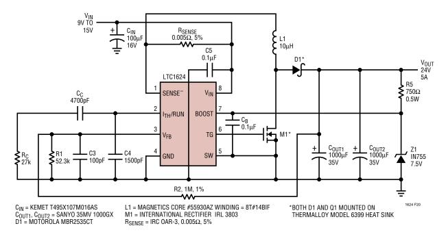
Figure 20. 12V to 24V/5A Boost Converter
