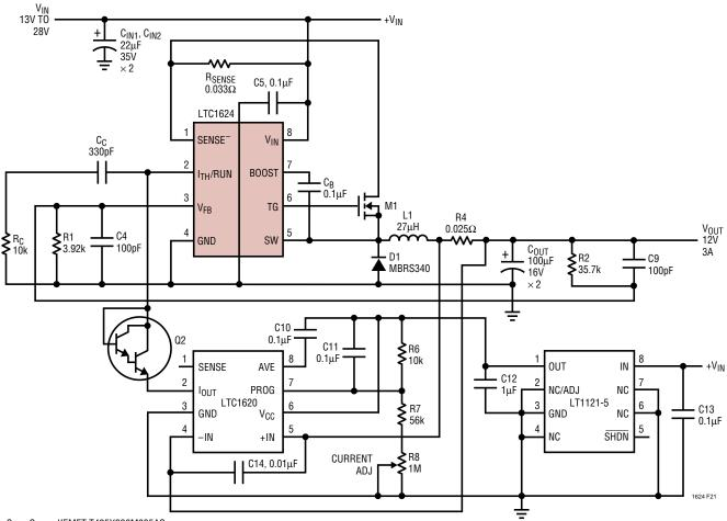
C<sub>IN1</sub>, C<sub>IN2</sub> = KEMET T495X226M035AS L1 = SUMIDA CDRH127-270 R<sub>SENSE</sub> = IRC LR2010-01-R033-F R4 = IRC LR2010-01-R025-F M1 = SILICONIX SI4412DY Q2 = MOTOROLA MMBT A14
