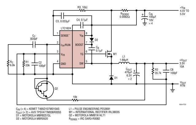
Figure 23. 5V to 3.3V/10A Converter (Surface Mount)
