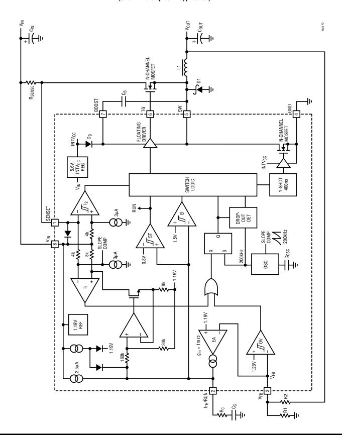
The LTC1624 can be used in a wide variety of switching regulator applications, the most common being the step-down converter. Other switching regulator architectures include step-up, SEPIC and positive-to-negative converters.
