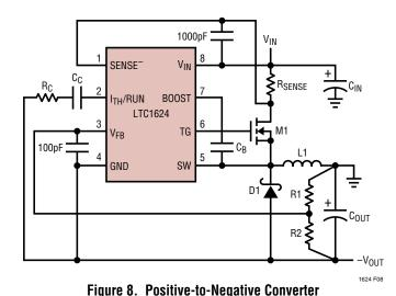
Positive-to-Negative Converter: Output Voltage Programming
