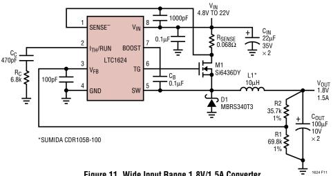
Figure 11. Wide Input Range 1.8V/1.5A Converter
