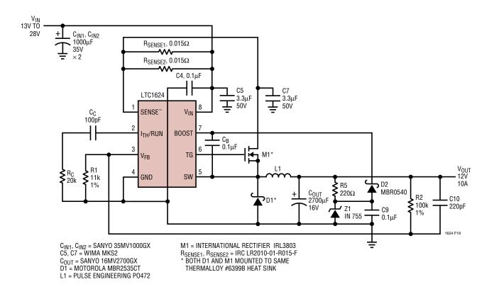
Figure 18. 24V to 12V/10A Buck Converter with Output-Derived Boost Voltage
