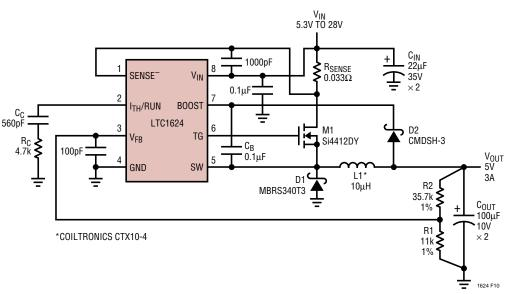
Figure 10. 5V/3A Converter with Output Derived Boost Voltage
