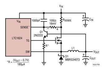
Figure 5. Modifying Burst Mode Operation
