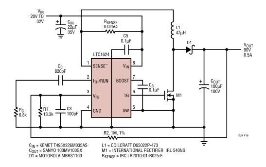
Figure 19. 24V to 90V at 0.5A Boost Converter
