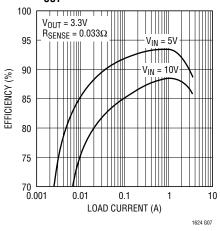
**Efficiency vs Input Voltage**  $V_{OUT} = 3.3V$
