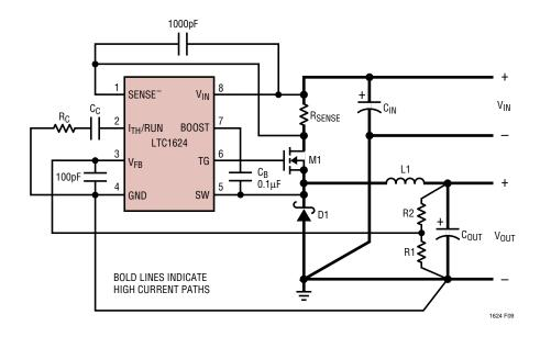
Figure 9. LTC1624 Layout Diagram (See Board Layout Checklist)
