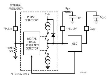
Figure 8. Phase-Locked Loop Block Diagram
