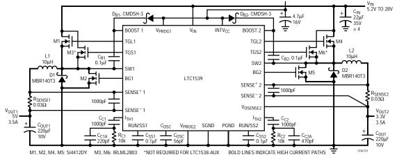
Figure 1. High Efficiency Dual 5V/3V Step-Down Converter
