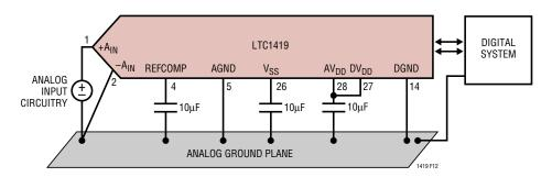
Figure 12. Power Supply Grounding Practice
