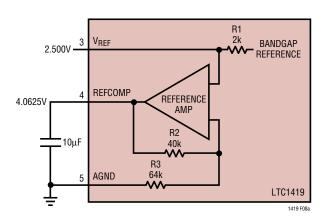
Figure 8a. LTC1419 Reference Circuit
