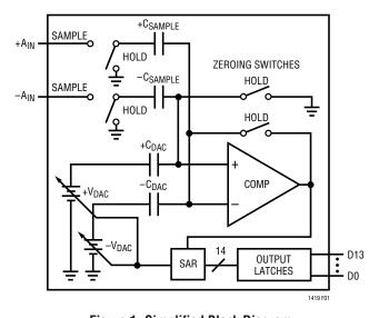
Figure 1. Simplified Block Diagram
