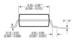
NOTE: DIMENSIONS ARE IN MILLIMETERS
