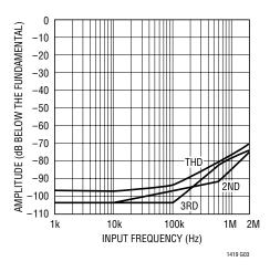
Figure 4. Distortion vs Input Frequency
