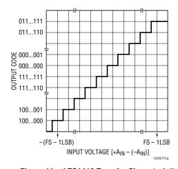
Figure 11a. LTC1419 Transfer Characteristics
