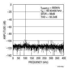
Figure 2a. LTC1419 Nonaveraged, 4096 Point FFT, Input Frequency = 100kHz
