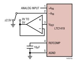
Figure 10b. Selectable OV to 5V or  $\pm 2.5$ V Input Range
