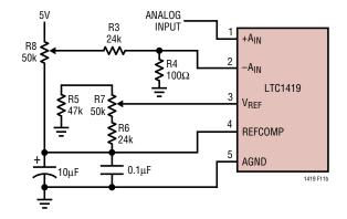
Figure 11b. Offset and Full-Scale Adjust Circuit
