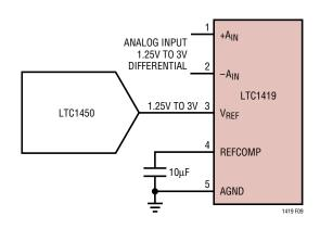
Figure 9. Driving V<sub>REF</sub> with a DAC
