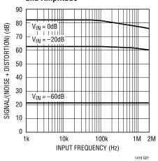
Signal-to-Noise Ratio vs Input Frequency
