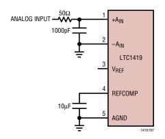
Figure 7. RC Input Filter
