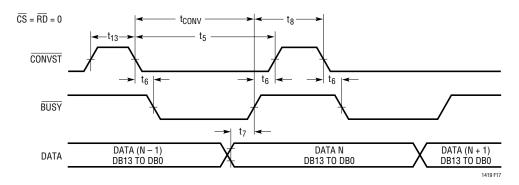
Figure 17. Mode 1b.  $\overline{\text{CONVST}}$  Starts a Conversion. Data Outputs Always Enabled ( $\overline{\text{CONVST}} = \boxed{\boxed{}}$ )
