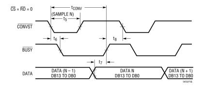
Figure 16. Mode 1a. CONVST Starts a Conversion. Data Outputs Always Enabled (CONVST = \( \bigcap \) \( \bigcap \)
