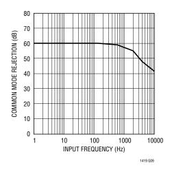
Figure 10a. CMRR vs Input Frequency
