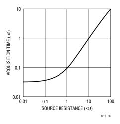
Figure 6. t<sub>ACQ</sub> vs Source Resistance
