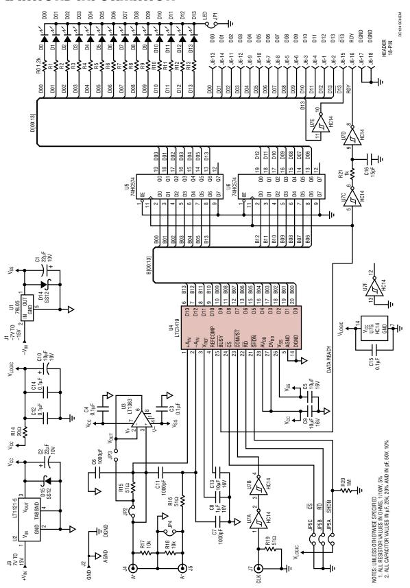
Figure 13a. Suggested Evaluation Circuit Schematic
