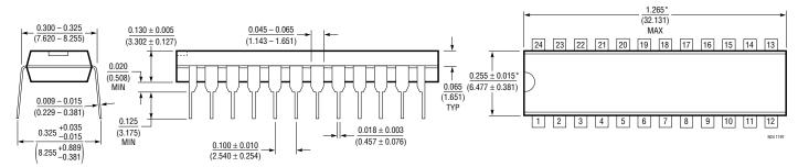
\*THESE DIMENSIONS DO NOT INCLUDE MOLD FLASH OR PROTRUSIONS.
