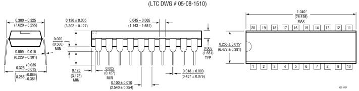
\*THESE DIMENSIONS DO NOT INCLUDE MOLD FLASH OR PROTRUSIONS. MOLD FLASH OR PROTRUSIONS SHALL NOT EXCEED 0.010 INCH (0.254mm)
