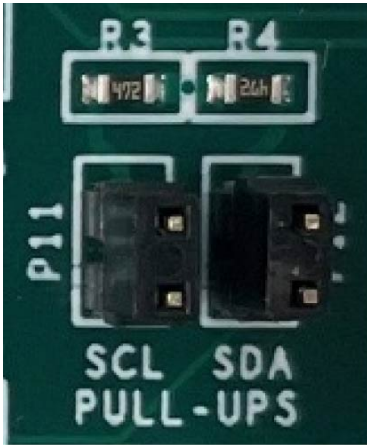
Figure 3. Selectable I 2 C Pull-Up Resistors
