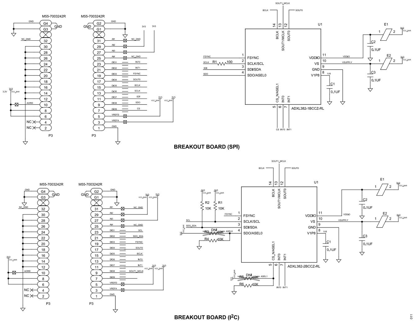
Figure 11. EVAL-ADXL380-BB-1Z or EVAL-ADXL380-BB-2Z Breakout Board Schematic
