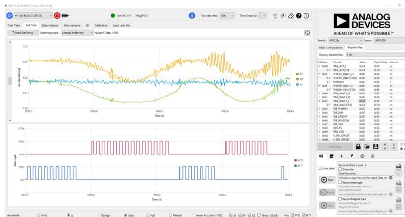
Figure 7. Activity and Inactivity Detection
