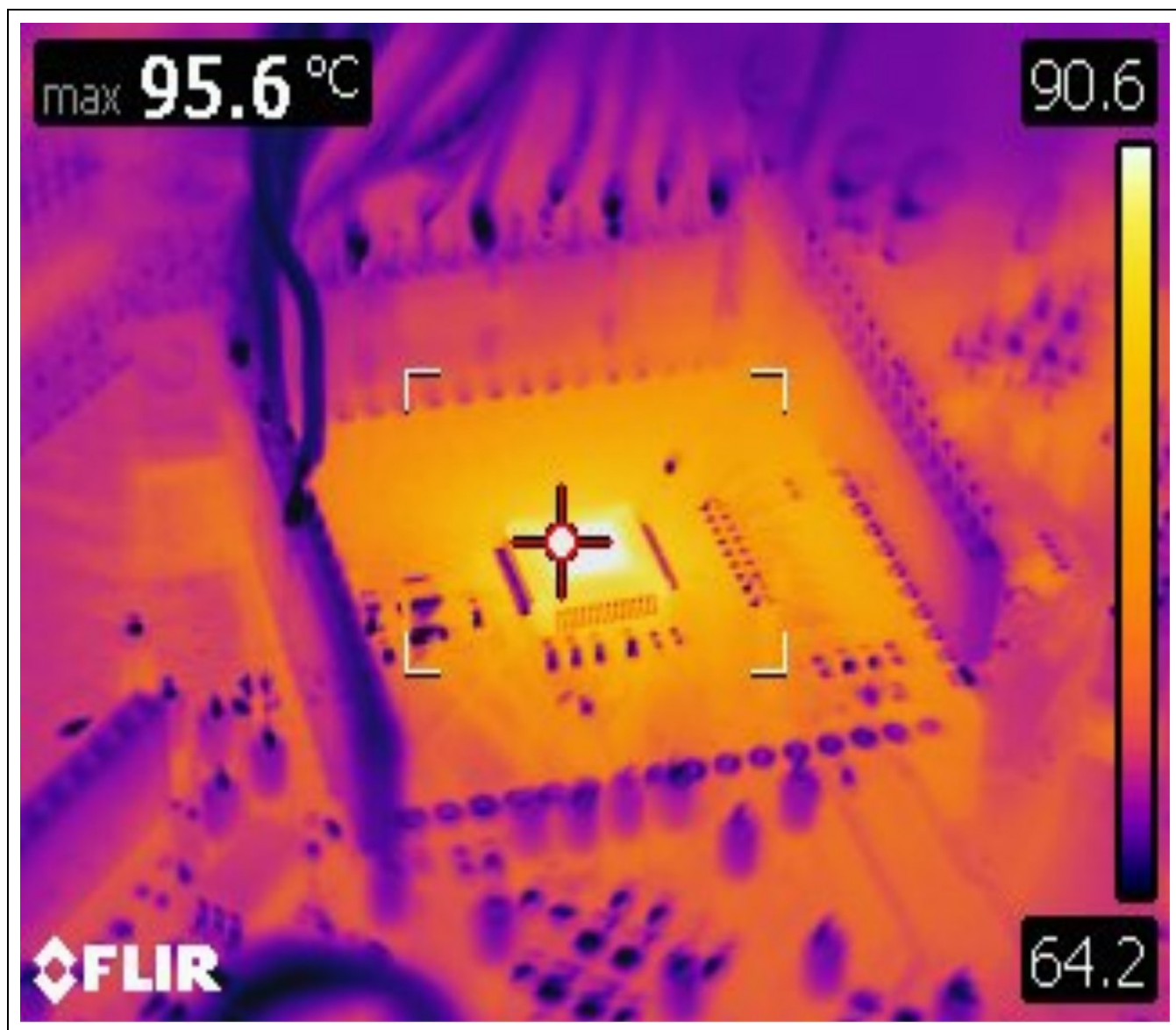
Figure 45. Thermal Image During Balancing of 7 Cells, 300mA, +60°C Ambient
