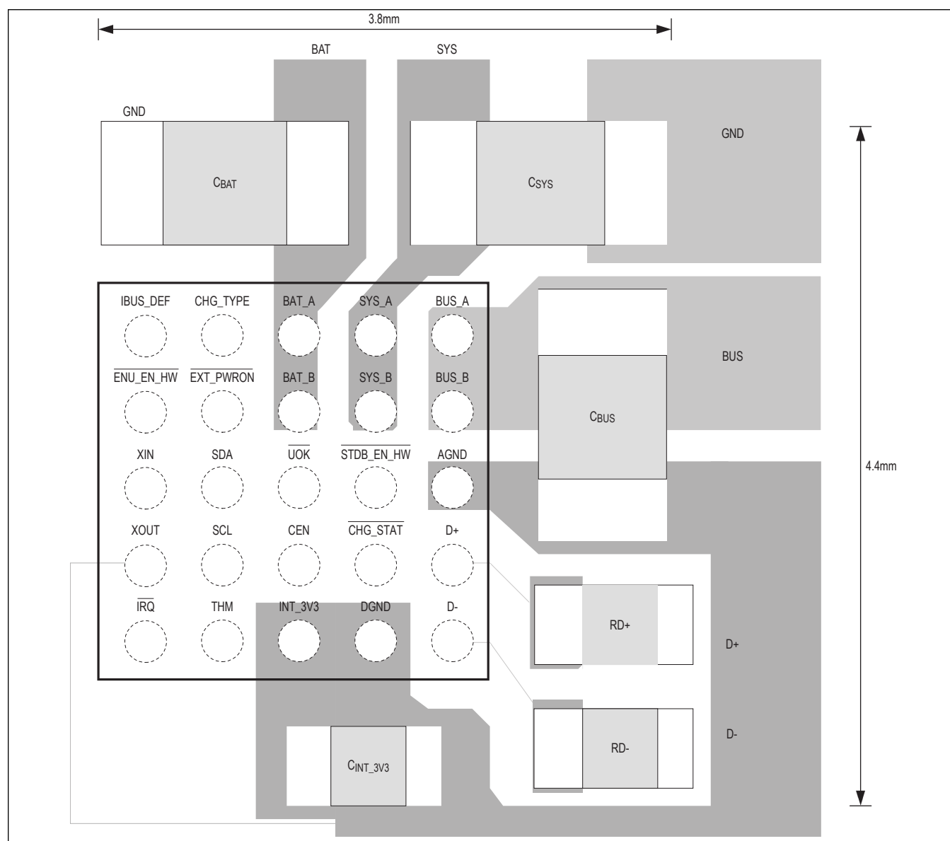
Figure 27. Recommended PCB Layout for Low Speed
