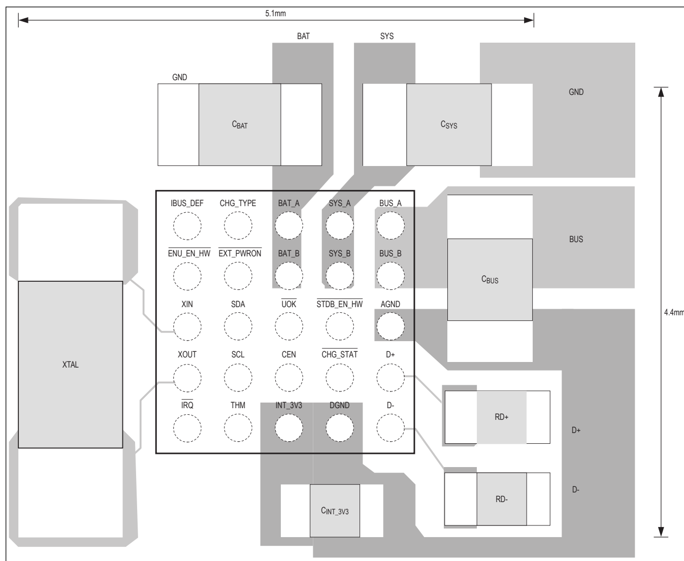
Figure 26. Recommended PCB Layout for Full Speed
