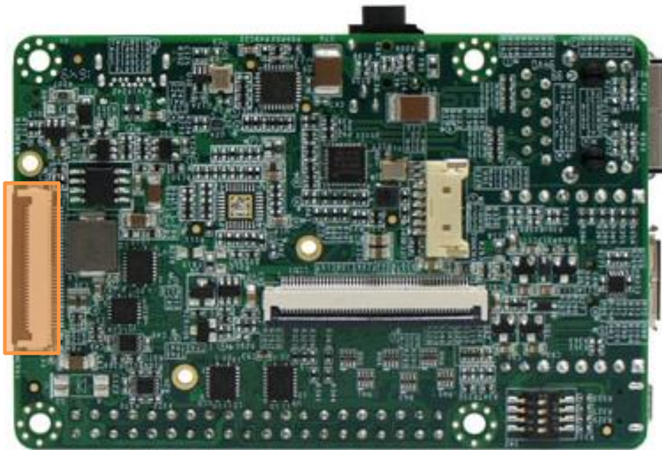
Figure 24 - PICO-PI-IMX7 Touch Panel Connector Location
