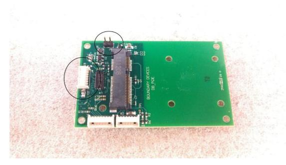
SABRE Lite/BD-SL-i.MX6. The cable must be plugged in with the orientation below, and requires a jumper to be installed.
