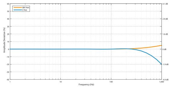
Note that the Slam Stick C has a DC response accelerometer (can measure down to 0 hertz). The plot only goes to 1 Hz because it is on a logaritmic scale. This data was generated with the sample rate at 3.2 kHz, and the unit taped to the mounting fixture.
