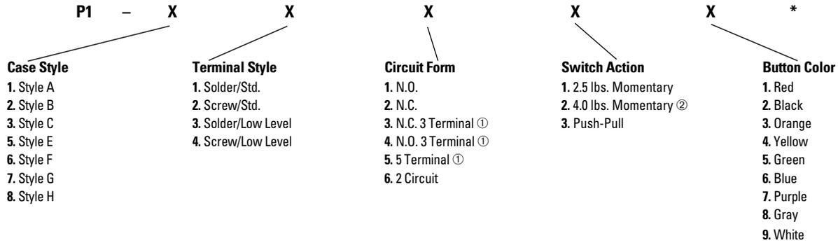
\* Add "W" for watertight to IP68S. (For watertight seal to MIL-PRF-8805 Design 3, please contact factory.)
