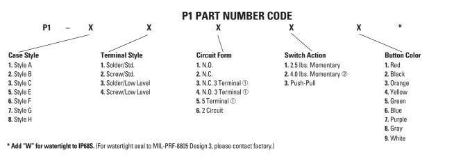
$\odot$  Circuit styles with 3 and 5 terminals have 50,000 cycle mechanical life per MIL-PRF-8805.  $\circledcirc$  Military standard is 4.0 lbs.
