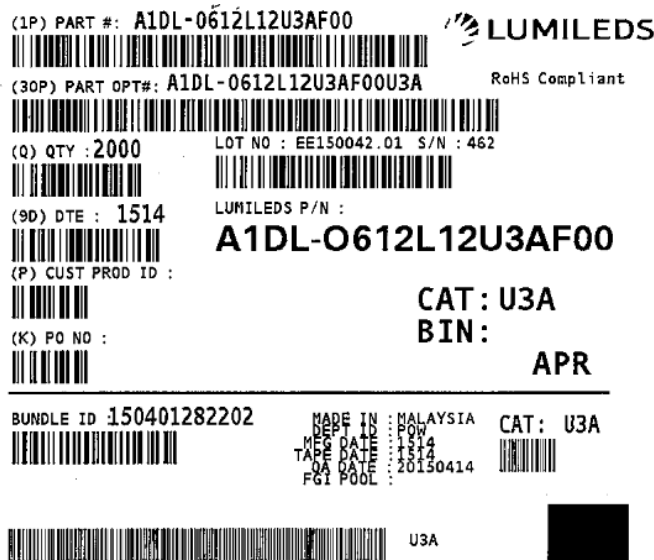
Figure 13. Example of a moisture barrier bag label.
