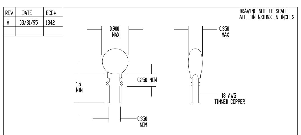
SPECIFICATIONS: RESISTANCE AT 25 DEG C = 2 DHMS +/- 15% MAX CONTINUOUS CURRENT (Imax) = 18 AMPS RESISTANCE AT Imax = 0.03 DHMS NOMINAL MAX VOLTAGE RATING = 265 VAC (RMS) MAX SURGE RATING = 80 JOULES ENCAPSULATION = SILICONE RESIN MARKING = OPTIONAL LEADS = RODAN P/N STL-209-45
