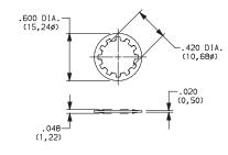
Pushbutton: 8700 Series Rotary: F Series Fits 5/16 Dia. Thread
