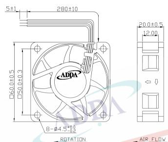
LEAD WIRES: UL 1007, AWG26, L = 280 ± 10 mm
