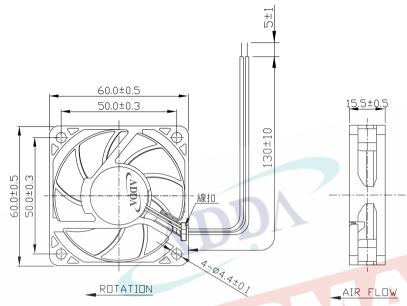
LEAD WIRES: UL 1007, AWG26, L = 130 +/- 10 mm Red = positive; Black = negative.
