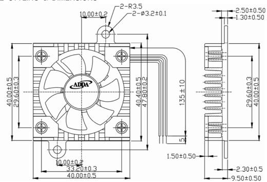
LEAD WIRES : UL 1571, AWG28, L = 135 + -10 mm Red = positive; Black = negative.
