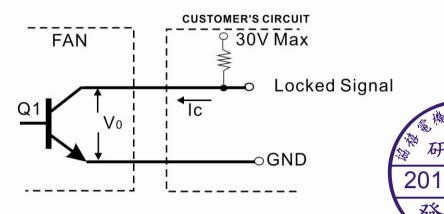
\*Transistor Q1 at "ON" position
