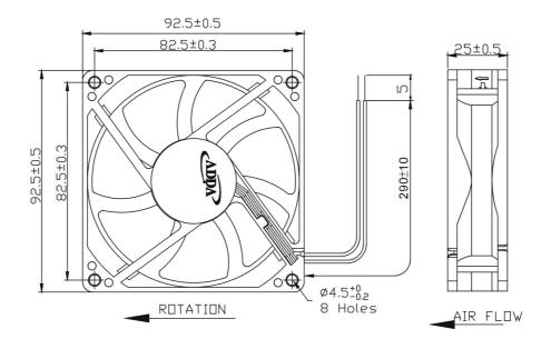
LEAD WIRES: UL 1007, AWG24,  $L = 290\pm10$  mm Red = positive; Black = negative.
