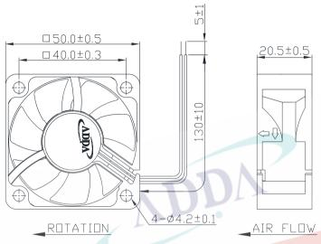
LEAD WIRES: UL 1007, AWG26, L = 130 +/- 10 mm Red = positive; Black = negative.
