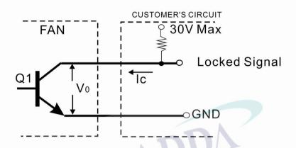
\*Transistor Q1 at "ON" position
