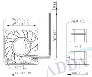
LEAD WIRES: UL 1007, AWG24, L = 310 +/- 10 mm Red = positive; Black = negative.
