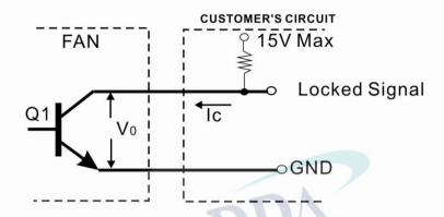
\*Transistor Q1 at "ON" position
