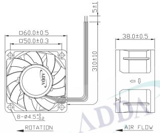
LEAD WIRES: UL 1007, AWG24, L = 310 +/- 10 mm Red = positive; Black = negative. White = FG
