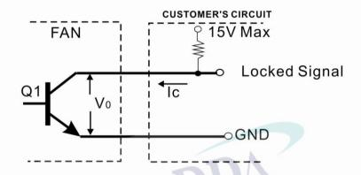
\*Transistor Q1 at "ON" position
