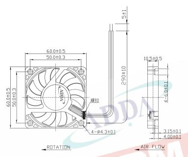
LEAD WIRES: UL 1007, AWG26, L = 290 +/- 10 mm Red = positive; Black = negative.
